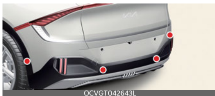
Ultralydsensorer bak (Type C-GT)
